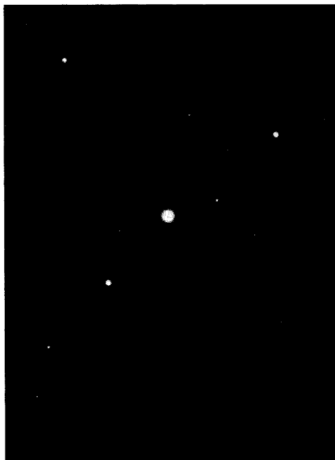
FIG. 4. Selected-area electron diffraction pattern of coke islands formed by methane on Ni, showing a near graphitic structure.
